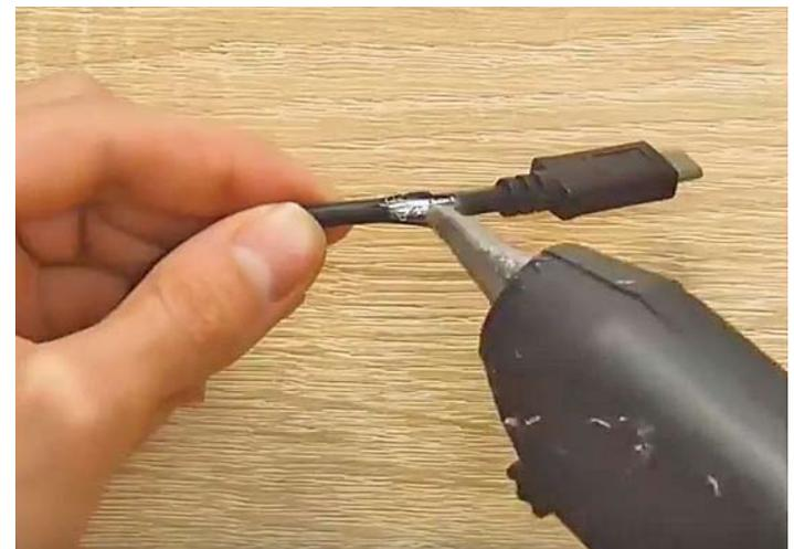
If the wiring on an electrical cable, such as on a corded drill, is worn or frayed, use a glue gun to seal the break. First, make a thin layer, let it cool completely. Add another larger, thicker layer on top of that layer.
