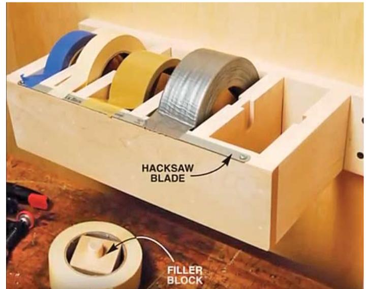
Instead of having all your tape (duct, blue painter's, wide masking tape, etc.) all scattered in a box or drawer, just build a tape dispenser like the one pictured above. Use a 12 inch hacksaw blade as a tape cutter. It already has two holes on each end to nail into the wood.
