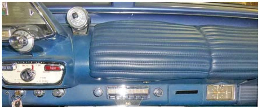
To the right of the instrument cluster is a padded dash. Right above the radio is the glove box. The round gauge between the glove box and the dash is a factory option, a Driver’s Power Seat Position Memory dial.
