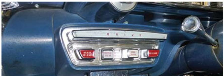
To start the car, turn the ignition switch to “on”, then hit the second button from the bottom left, it says “Neutral Start”. Once the car is running, press the wide top button that says “Drive”. Reverse is the red button on the bottom right. The far left bottom button is for the “Brake Release”. The third button from the bottom left is “Hill Control” for engine braking on steep grades.
