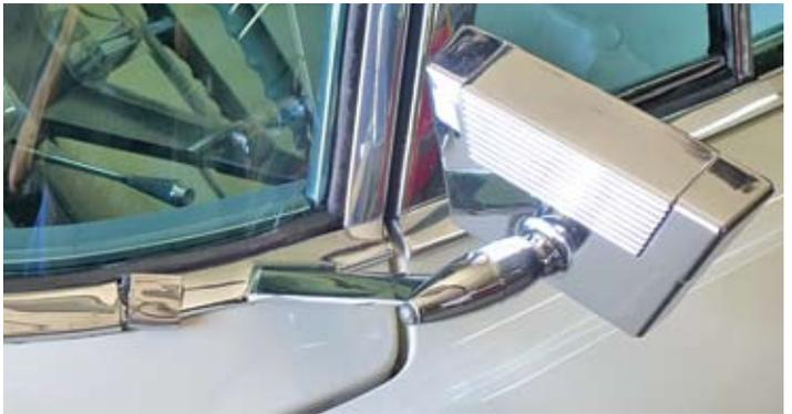
The driver's side outside rear view mirror is mounted to the body and not to the door.
