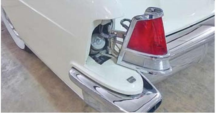
The driver's side rear turn signal swings away to reveal the hidden gasoline filler tube.
