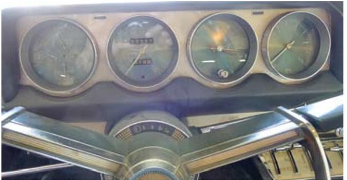
The instrument panel has four large circular faces. The far left (4 gauge) cluster houses the fuel level, water temperature, oil pressure and amperage gauge. The speedometer and odometer is to the right. To the right of that is a clock. The far right gauge is an engine tachometer reading up to 5,000 rpms.
