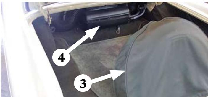
The “tire bulge” on the trunk lid is for a near vertically mounted spare tire (arrow # 3). The trunk space is wide but not very deep due to
