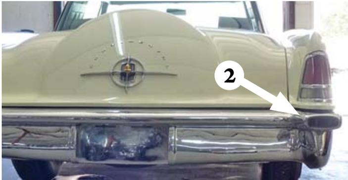
The front bumper has built in rectangular turn signals (arrow # 1) which are replicated in the rear bumper as small rectangular exhaust ports under the rear turn signals (arrow # 2).
