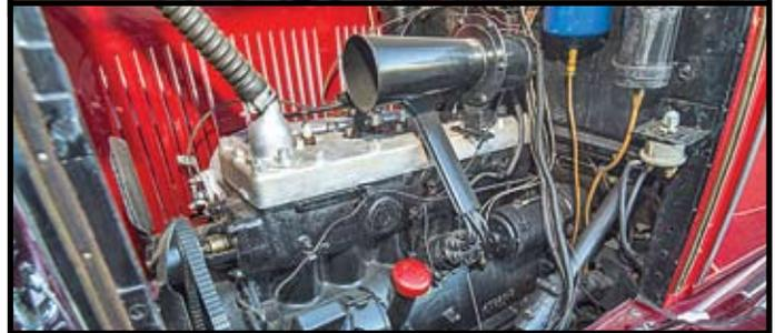
" 175 CI inline 6-cylinder engine, Stromberg carburetor, 3-speed manual transmission
