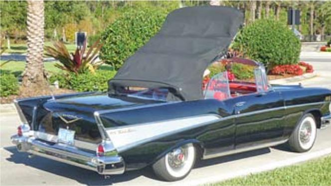
The drivetrain is all original and numbers matching. The 265 cubic inch V-8 engine was rebuilt recently by Gene's Repair Shop in Casselberry, FL due to an excessive oil burning issue. Steve is very happy with the repair. The 4 barrel carburetor was also professionally restored by a Florida carburetor shop. The two-speed Powerglide automatic transmission remains untouched since Steve bought the car.
