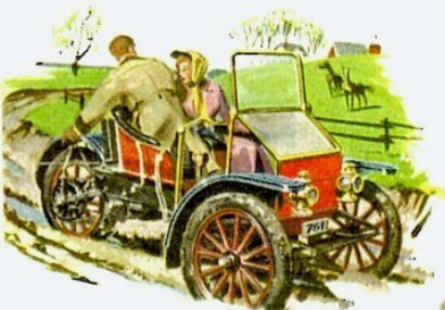
1911 KELSEY was a little three-wheeler that sold for $385. It was light and easy to handle, and its two-cylinder engine drove it only 25 miles per hour.
