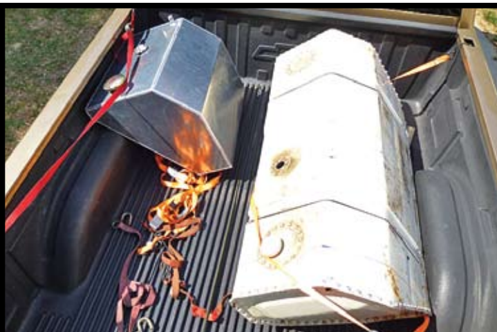
The new fuel tank (left) next to the old one.
