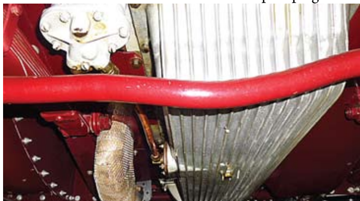
The 40 inch long oil pan holds up to 12 quarts of motor oil !
