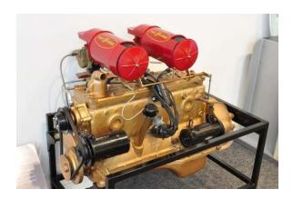
Hudson offered a variety of six and eight-cylinder inline L-head engines over the Step-Down's seven production years, but the most famous of the bunch was the H-145 Hornet six introduced in 1951. Based on a high-chromium alloy block, the Hornet displaced 308 cubic inches—relatively enormous for a straight six at the time—and was offered in standard 145 hp form and in optional Twin-H tune with twin Carter WA-1 carburetors and an initial rating of 160 hp.
