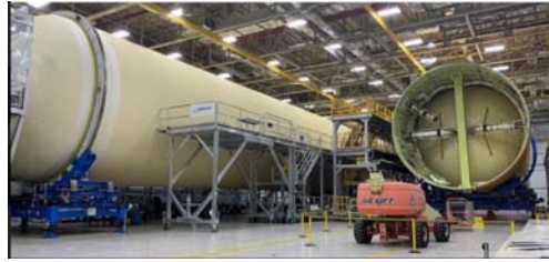
Core Stage LH2 fuel and LO2 oxidizer tanks at Michoud assembly
