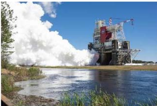
Artemis I core stage green run test in the B-2 test stand at NASA's Stennis Space Center. Credits: NASA
