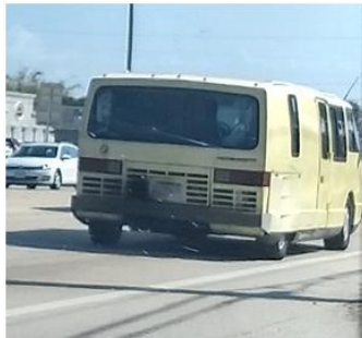
Seen March 9, 2019 on Highway A1A Cape Canaveral – Vivix BMW RV has an exceptionally low center of gravity and wide stance for an RV. It had a top speed of 100 MPH, and claimed an average of 30 MPG using a BMW M21 turbo-diesel engine
