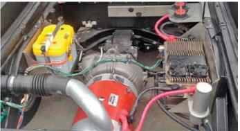
Rotisserie restored, Electric Powertrain with Netgain WarP 11 DC motor, 120 CI electric engine, Silver paint, Silver leather bucket seats, Wilwood disc brake conversion Powdercoated running gear, Air conditioning, Power windows, Line-X bed liner, Soliton 1 controller Manzanita onboard charger MiniBMS battery monitoring 63 Lithium batteries 3.2 V each wired in series for total of 202 V Bluetooth generated touch screen power monitoring system
