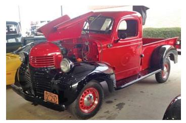
Flathead 6-cylinder engine 3-speed manual transmission 6 volt system Crank-out front windshield Wood bed floor
