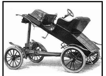
The uniqueness of the Phelps, The body can be lifted to expose the chassis and engine for easy maintenance.
