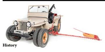
This 1946 Willys CJ–2A farm Jeep has a front PTO winch and engine driven air compressor. It has a welding unit in the passenger seat area, and a side arm mower bar on the driver's side. It also has a rear towing boom and a Newgren buzz saw with table. The dual tires front and rear provide stability and traction when in the dirt.
