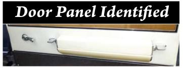
This door panel with two interior door release levers is from a **1963 Buick Riviera**.
