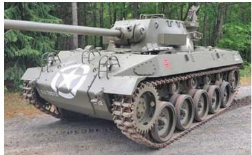
This vehicle was restored from an empty hull in 2012-2013. It has the more powerful R-975 C4 motor which makes it the fastest most powerful WWII tank you will drive. The motor was rebuilt in 2013 as well and runs perfectly. The tank has a little joe generator which is fully functional as well as a functional turret motor. Gun is not live, and the breech has been demilled.
