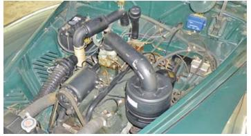
An oil bath air filter in the large black canister is attached to the 2 barrel downdraft carburetor.
