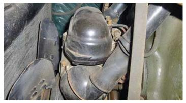
Here's the distributor mounted at the front of the engine about a half inch behind the metal radiator fan. There are 6 spark plug wires going to each side of the distributor. There are 2 coil assemblies used for each side of the engine. If you have a 1942 Ford flathead V–8 engine, then this setup will look familiar to you.
