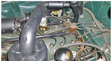
There are 6 spark plug wires feeding into a metal tube, on each side of the engine, that goes to the distributor at the front of the engine. There is plenty of room in this engine compartment to work on this engine.
