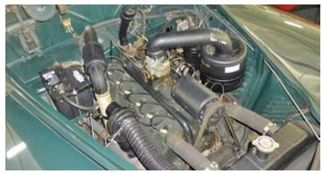
A 6 volt battery starts this small V–12. The dual radiator hoses to each cast iron head is similar to a 1942 Ford V–8.
