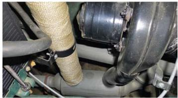
The driver's side exhaust manifold goes underneath the engine's oil pan and connects to the passenger side
