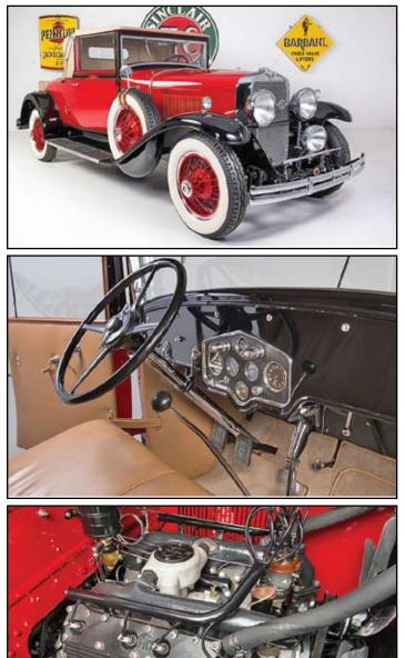
"This (2008 AACA Senior and) concours winning **LaSalle** is equipped with a V–8 power plant, 3-speed synchromesh transmission, wire wheels, dual side mount spare tires, Pilot Ray driving light, radiator stone guard, rumble seat, rear mounted trunk and golf bag door".
