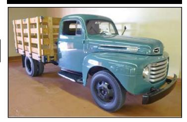
In September 2013, I saw this **1949 Ford F–4 Stake Bed Truck** with less than 56,000 original miles (2 owners, 1 repaint) at a south Orlando car dealer's showroom. It was for sale for \$15,900. It has a 226 cubic inch (3.7 liter) inline flathead six cylinder engine with 95 horsepower at 3,300 rpms. It has a 4 speed manual transmission. It's a heavy duty no frills 2 wheel drive work truck.
