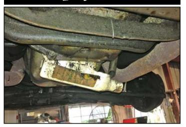
In September 2013, while visiting Gene Roy's Car Repair Shop in Casselberry, FL, I came across this low cost way to control a car's oil leak. On this **1958 Packard** on the car lift, the owner installed a cut up plastic oil bottle under the bellhousing to catch a slow oil leak. He bolted the side of a plastic oil bottle to two lower bellhousing bolts. Since the bottle is installed at a slight downward angle, the owner can unscrew the bottle top to drain the accumulated oil.
